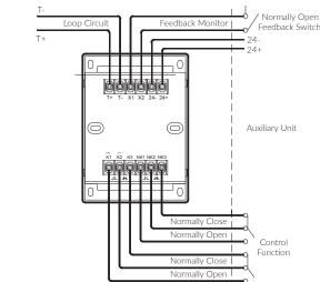
There are ten connecting terminals mounted on the printed circuit board. Terminals T+ and T- are utilized for loop circuit wiring, terminals X1 and X2 are used to connect to a normally open feedback line input for monitoring and terminals K1 to NK3 are relay contacts wherein K1-K2 & NK1-NK2 are normally Open contacts and K2-K3 & NK2-NK3 are normally Close contacts.
