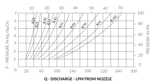
Q = K $\sqrt{P}$  where P is supply pressure in Kg/sq.cm., K= nozzle constant (K-factor) in metric US K factor = Metric K factor MK ÷ 14.2745
