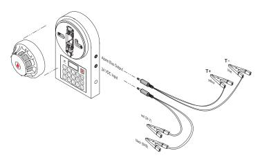
The LF-DP-6190 Handheld Programmer can be used either by installing a detector through its fascia or through alligator clips depending on the type of bus equipment. The first set socket terminal on the right side (yellow, blue lines) is the Alarm Bus Output Line which is used for address coding and analog value operation reading. The second set socket terminal (red, Black lines) is 24 V Power Supply Input Line which is used when the programmer uses external power supply.
