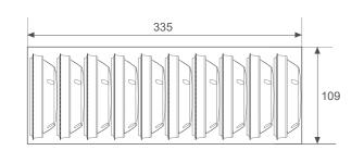
•Carton box - 100 units S30, (10 master boxes), no bases included, dimensions556 x 345 x 231 mm. All detectors are protected with a plastic cap.
