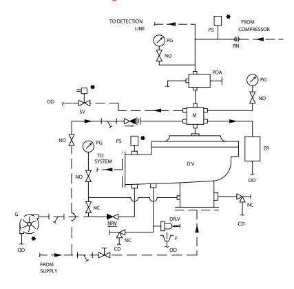
Electric & Hydraulic Release Trim - Schematic Deluge Valve Model - A Size 200 / 150 / 100 / 80 / 50 NB
