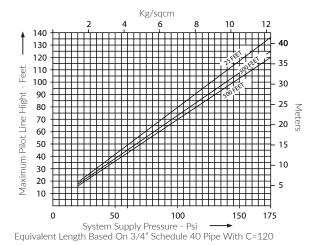
Wet Pilot Sprinkler Height Limitation of 150 NB
